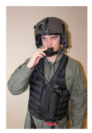
The SEA unit can be mounted in the front or back/side, left or right for best integration with the cockpit interior. Above the front mount is shown.
