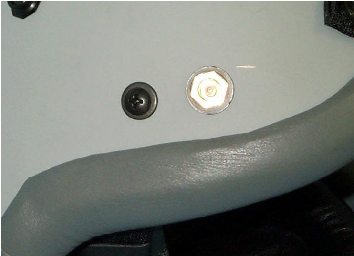
Figure 2. Close-up, showing location of the CEP connector in the HGU-55.
