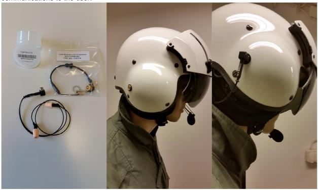
The CEP consist of a pair of mini-speaker elements combined with earplugs to provide a
